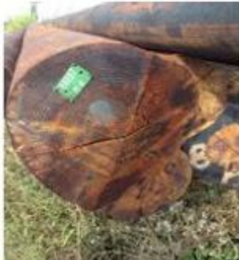
Typical Examples of Splits in Poles
