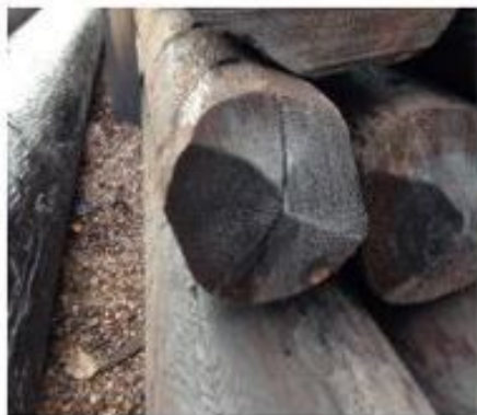
Typical Examples of Splits in Poles
