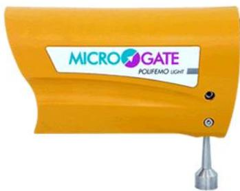
Rechargeable, single beam photocell. 15 meter optical range
