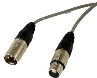
3 conductor 24 awg shielded cable 100 feet long, with XLR-3 male and female connectors.
