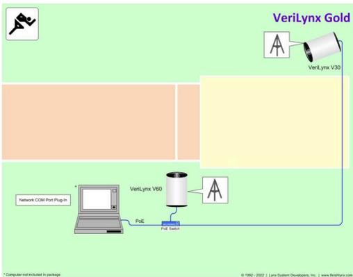
Includes 2x (camera, lens, tripod, PoE adapter, cables, carrying case), software, 5LNCP and PoE Switch
