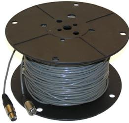
3 conductor 24 awg shielded cable, 500 feet long, with XLR-3 male and female connectors.
