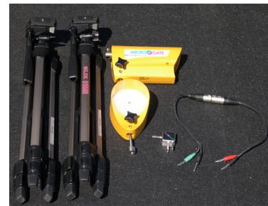
Includes two 15m range single beam photocells, two reflectors, two tripods and two double mounting supports and double photocell cable
