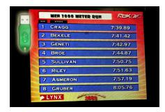
Broadcast version suppresses Lynx Logo. When Combined with a Scan Converter, allows Results and Running Time to be displayed dynamically to CCTV and other TV output display devices. Connects via network or serial port to any PC running FinishLynx.
