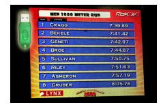
Configurable graphics application allowing results and running time data to be dynamically displayed on LED video screens, CCTV, and other TV devices via an HDMI output. Supports network or serial port to any PC running FinishLynx, FieldLynx or LynxPad.
