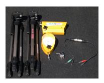
Includes two 15m range single beam photocells, two reflectors, two tripods and two double mounting supports and double photocell cable
