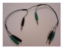
Allows two photocells to be connected in serial to produce one signal when both beams are broken
