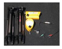
Includes one 15m range single beam photocell, one reflector, two tripods, mounting supports and photocell cable.
