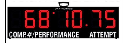
Alternates between three digits of competitor ID plus attempt number and performance in metric or imperial. Works with FieldLynx. Can also be used as a running time clock with FinishLynx or standalone.
