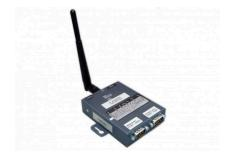
Allows wired or wireless communication to two serial devices on a LAN using TCP-IP mapping.
