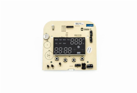
IOTMAX1 Geyserwise Max or Delta T PCB for TUYA retrofit
