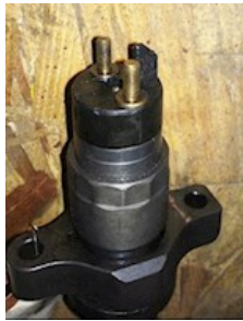
Damaged Dodge CR Injector
