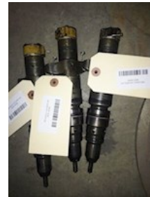
Damaged CAT C7/C9 Injector
