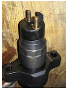
Damaged Dodge CR Injector
