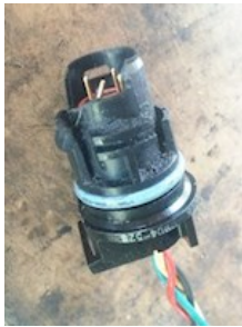
Damaged Ford 6.0 Injector Plug
