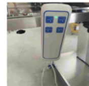
Wired positioning control
